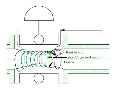
fluid is an insulator, conductor, or semi-conductor, and it isolates the I/O circuit from the wear-wire to protect sensitive SCADDA components.
