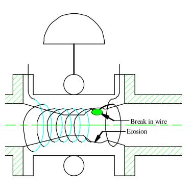
But this situation can get stickier: What if the piping in the plant is grounded (as it normally is)? In this case, when the wear-wire is exposed to the process fluid, the I/O electric potential is shorted directly to ground.
