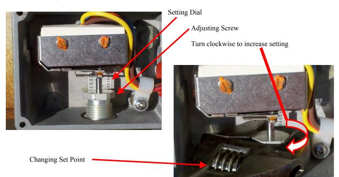
The set point on mechanical pressure switches is verified through a trail-and-error process that involves pressurizing the system and observing where the switch contacts actually transfer. This is usually accomplished by turning on the pump and throttling the discharge valve, gradually deadheading the pump until the switch trips.
