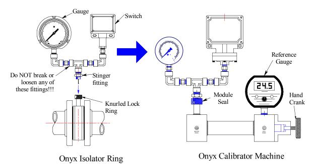
Gauges, switches, transmitters, or any combination of these instruments can be temporarily removed from the Onyx Isolator Ring, attached to the calibration machine for verification, then put back on the isolator ring. To calibrate the instrument, simply turn the crank to build up the required pressure and compare the reading of the process instrument to the reference gauge.
