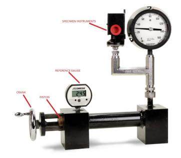
This rugged machine is light weight, portable, and requires no external power, making it ideal for field service. It can generate pressure from near full vacuum to +400 psi.
