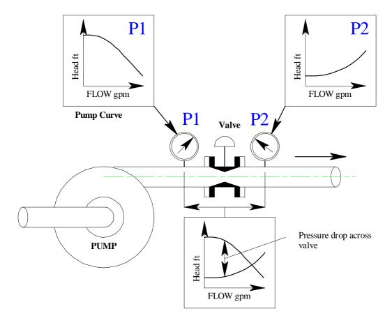
The inlet pressure is determined by the pump curve (or the tank head in a gravity system).
