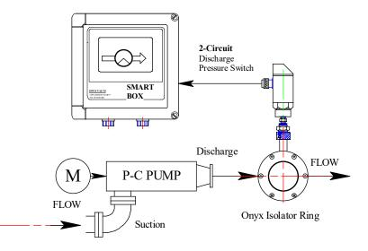
How can you protect a pump against **BOTH** Over-Pressure and Run Dry with 1 Switch?
