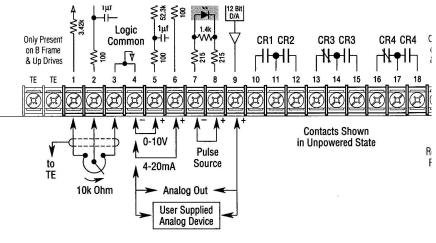
In our example we used CR-1 as the run relay. Connect terminal #10 in the A-B drive to Smart Box terminal #2. Connect terminal #11 in the A-B drive to terminal I-1 in the Smart Box.
