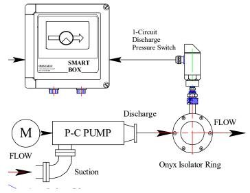
Protecting a pump against a **Run-Dry fault** is a little trickier. There are two ways to accomplish this:
