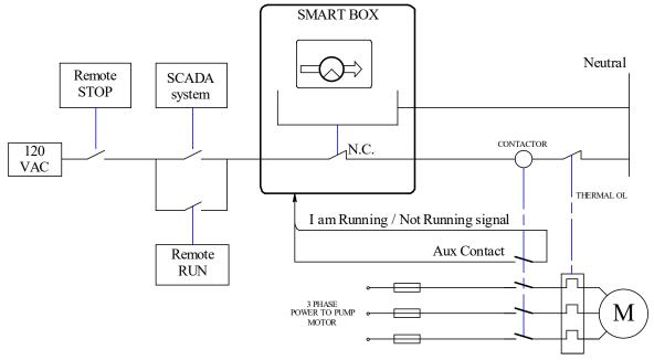
The Smart Box has a permissive contact O-1 that remains closed continuously whether the pump is running or not. This contact stays closed unless there is a problem. If there is a fault in the system, this contact opens until you fix the problem and press RESET on the Smart Box.
