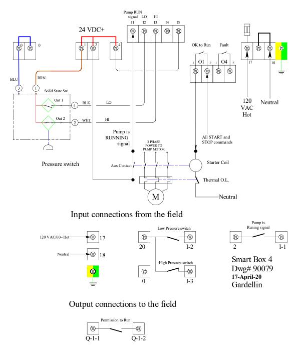
It is imperative that the Smart Box is the last link in the chain and that there are no other devices between the Smart Box and the starter coil that can start the pump. Output-4 is an optional "FAULT" signal that you can use to illuminate a remote FAULT light or to tell a supervisory SCADDA system that the pump is off-line because of a fault condition.
